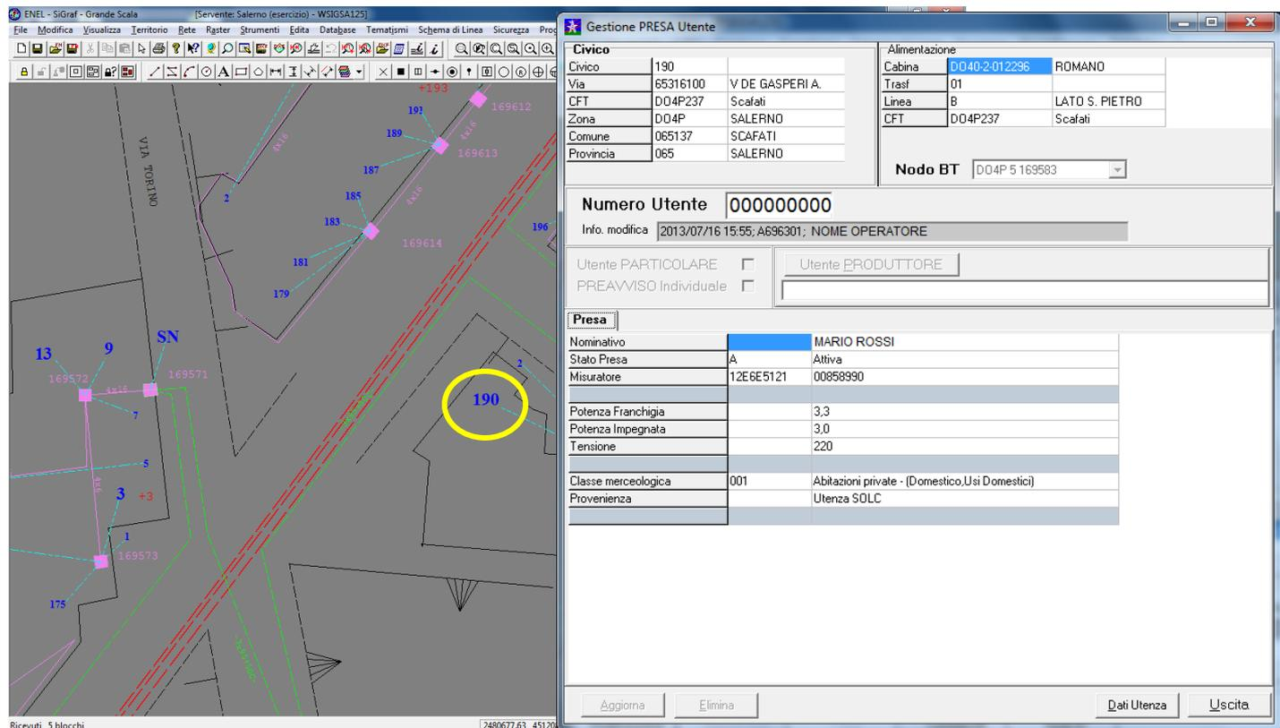
The screenshot displays the ENEL-SiGraf software interface. On the left, a map shows a network of lines and nodes. Node 190 is highlighted with a yellow circle. On the right, the 'Gestione PRESA Utente' window is open, showing details for user 190.
